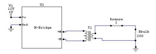
The onboard microprocessor requires reprogramming. The microprocessor will reverse the output every 1/60 of a second to simulate power line frequency. Wave shaping is possible however a square wave output and modified sine wave output are the easiest to construct. True sine wave output can be obtained with PWM and output filtering. One may also consider a slow turn routine to increase bulb lifetime.
